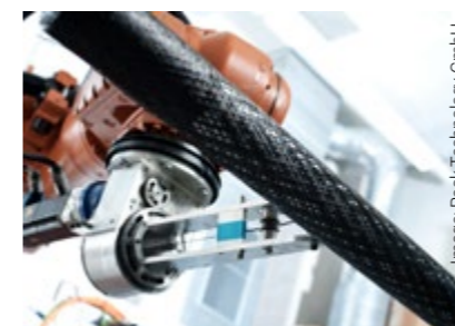
Automated winding process for manufacturing carbon fibre reinforced lightweight parts.
