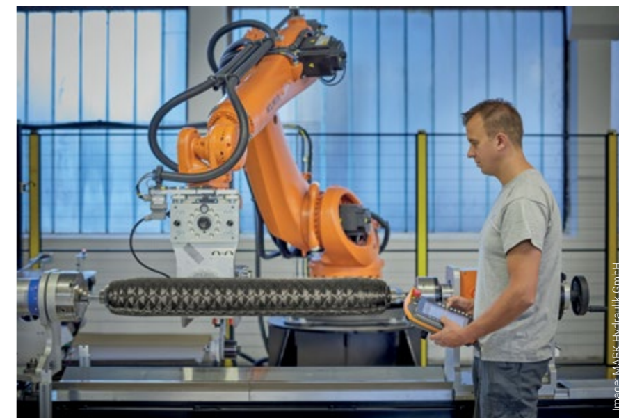
MARK produces ultra-lightweight, corrosion-free hydraulic cylinders.
