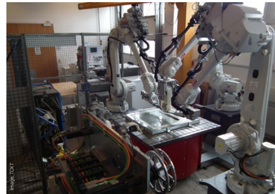
Automated tape laying
