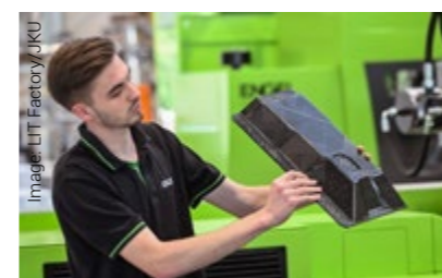
Combination of the ENGEL technologies organomelt and UD-Tapes in a demonstration part
