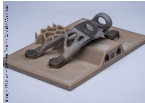
Image: TU Graz – IMAT/Hoflehner/Carvalho/Amanco Ultrasonic Joining of FFF-PEEK with LPBF 316L stainless steel
