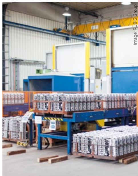
The innovative techniques of RUBIG Aluminum, including T4, T5, T6, and T7 treatments, employ varied quenching methods aimed at achieving unmatched strength, minimal distortion, and superior toughness.
