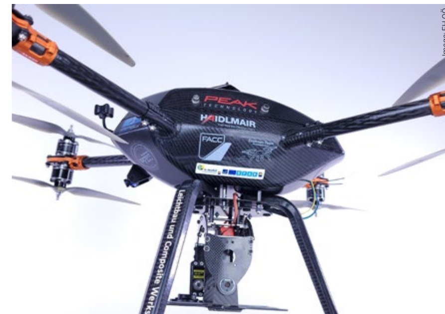
Weight-saving, high-strength composites are the ideal material for drones. Students at the University of Applied Sciences Upper Austria applied their know-how and expertise in lightweight design to develop a camera drone in a very integral design and enable a weight saving of more than 40 %.
